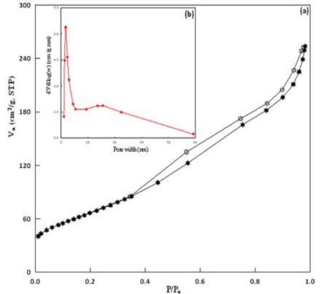
Fig.2.  $N_2$  adsorption-desorption isotherm (a) and pore size distribution (b) of GMC sample
