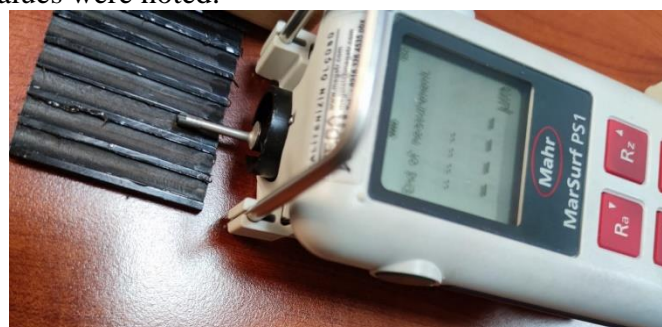
Fig. 1 Roughness Measurement Setup for UHMW
