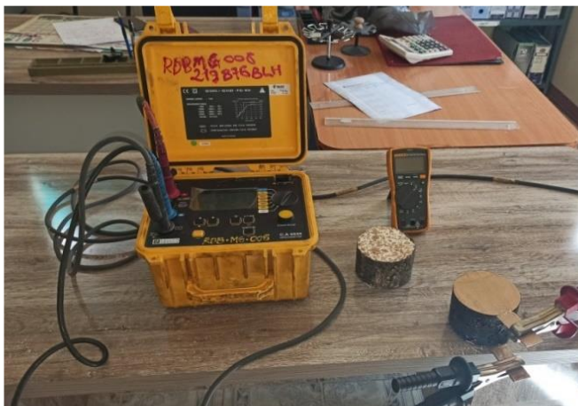
Fig. 1 The two-point method to measure electrical resistance
